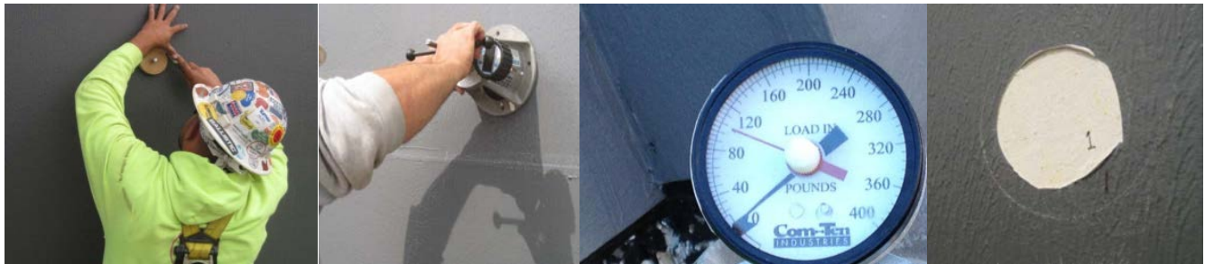
ASTM D4541 test apparatus and photos – for reference only
